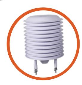
**AR300-19 CH4 concentration sensor** adopts the catalytic combustion principle and has a built-in high-sensitivity probe. It has the characteristics of high accuracy, good linearity, and easy installation. It is widely used in industrial plant, traffic tunnel, coal mine shaft, dig working face, dye stuff plant, warehouse storage, chemical plant, etc.
